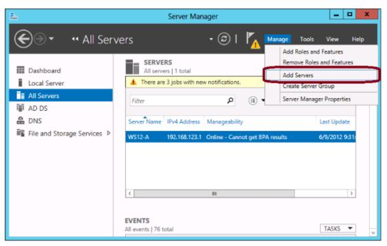
FIGURE 1-4 Adding a remote server to manage in Server Manager.
